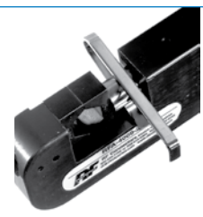
Lower die removal
